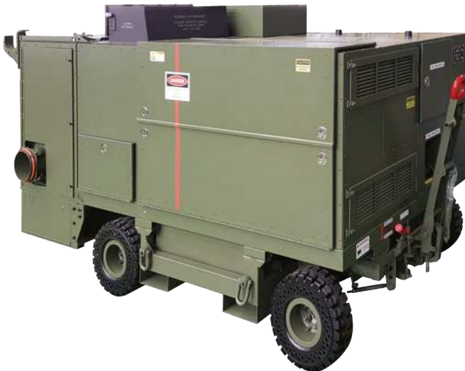
GTGA (Gas Turbine Generator, Combined Air-conditioner)
