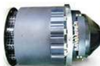
60KW 120/208VAC, AC60KW 2,400~8,000RPM BRUSHLESS TYPE ø 270 x L430, 55KG
