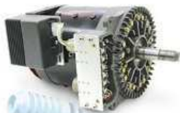
KAAV 300A 28VDC, 300A, 2,400~8,000RPM BRUSHLESS TYPE ø 250 x L3773, 35KG
