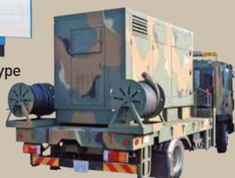
Generator Set Truck
