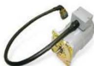
Motor for arm turn 24VDC, 880W, 2,200RPM under 55Arms
